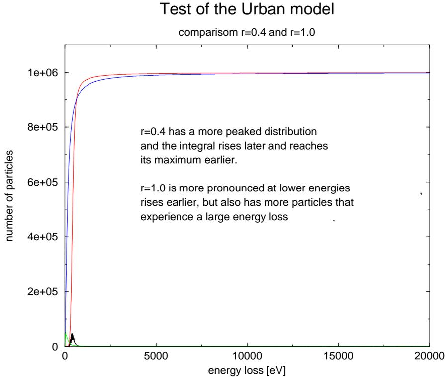
Figure 5: The integral of the curves in Fig. 4 shows the number of particles which encountered energy loss less than the value on the abscissa.
