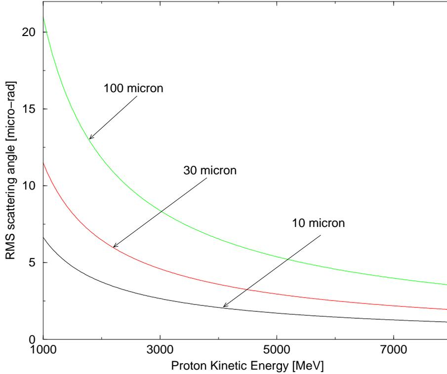
Figure 2: *Transverse scattering angle as a function of beam energy for pellet diameters of 10, 30, and 100  $\mu\text{m}$ . This case is relevant for HESR.*
