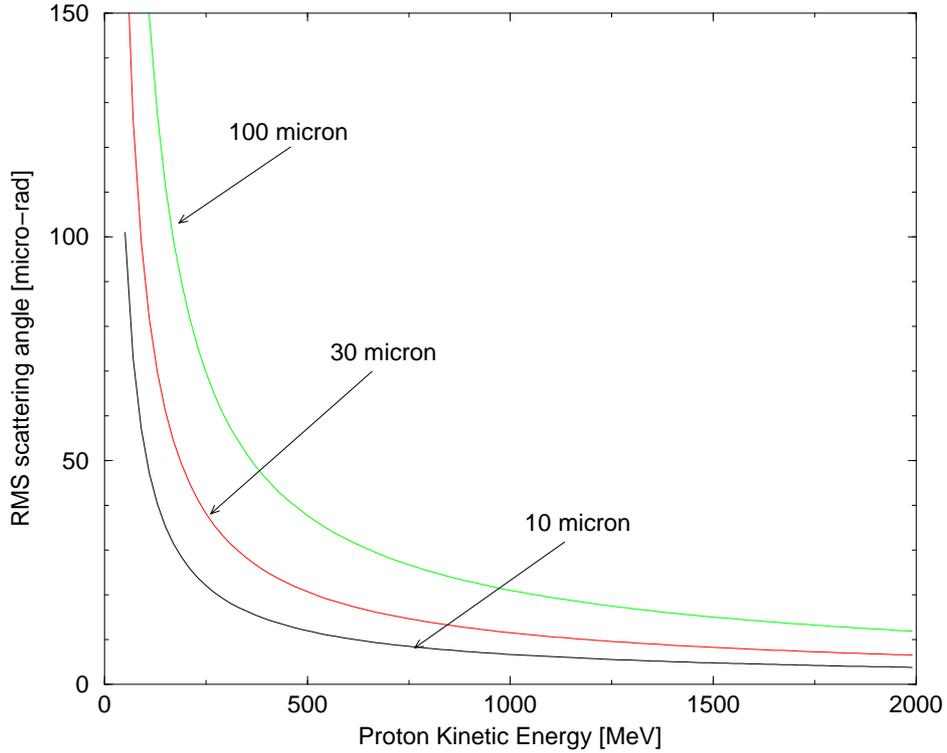
Figure 1: *Transverse scattering angle as a function of beam energy for pellet diameters of 10, 30, and 100  $\mu\text{m}$ . This case is relevant for CELSIUS.*
