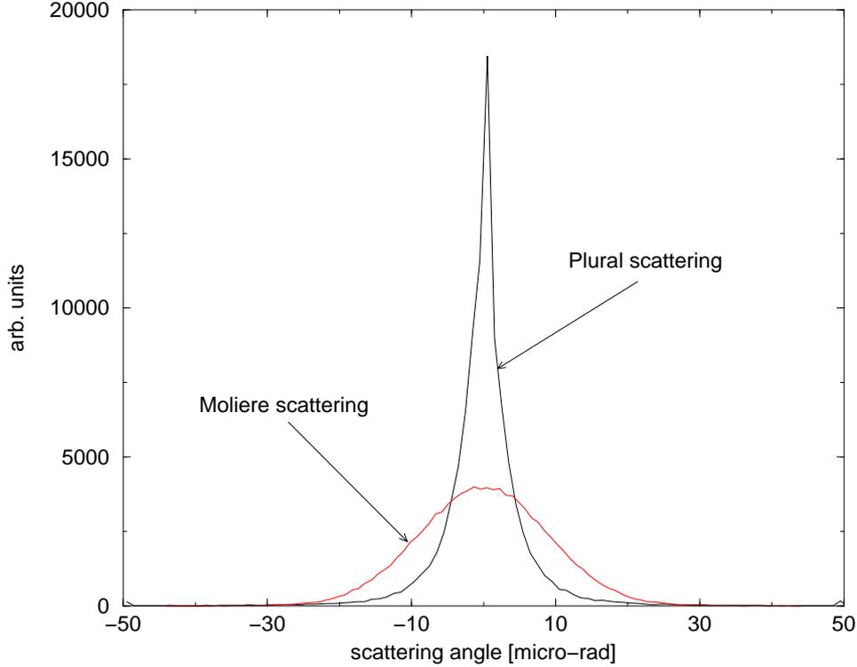
Figure 3: *Molière versus plural scattering for 1360 MeV protons scattered off pellets with 30  $\mu\text{m}$  diameter.*
