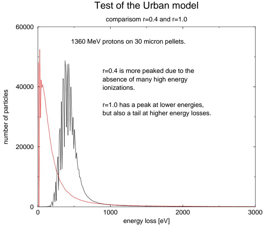
Figure 4: *Energy loss distribution for 1360 MeV protons impacting on 30  $\mu\text{m}$  pellets simulated by the Urbán model with parameter  $r = 0.4$  and  $r = 1.0$ . The curves are based on one million proton hits.*
